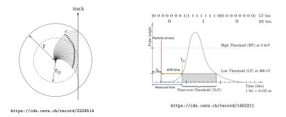
First electron drift time :  $t = t_{LE} - (t_{collision} + t_{ToF} + t_{SP}) = t_{LE} - T_0$
