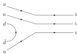
**Resonance** formation can happen when a meson is involved, and results in a single outgoing particle, for example  $p\pi^+ \rightarrow \Delta^{++}$  or  $\pi^+\pi^- \rightarrow \rho^0$ . The cross section for the formation of a particular resonance  $R$  is given by
