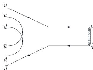
**Annihilation** occurs in baryon-antibaryon collisions when quark-antiquark pairs annihilate. Strings are formed between the remaining quark-antiquark pairs. Cross sections for annihilation are found by parametrization for  $p\bar{p}$ . For all other cases, the cross section is a rescaling of this value.
