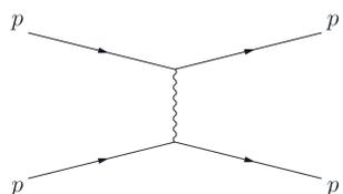
**Elastic** scattering refers to particles interacting and deflecting without changing their type. Elastic cross sections are calculated by interpolating data and using the CERN/HERA interpolation when available, and using the AQM model otherwise.
