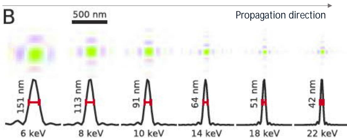
Measurement of the energy dependence of the focused beam size at NanoMAX
