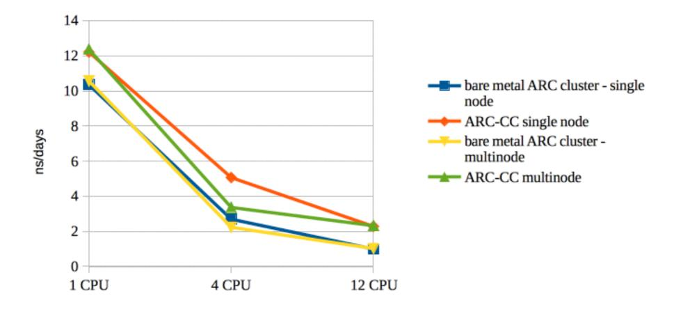
Days of computation time required per nanosecond of simulation
