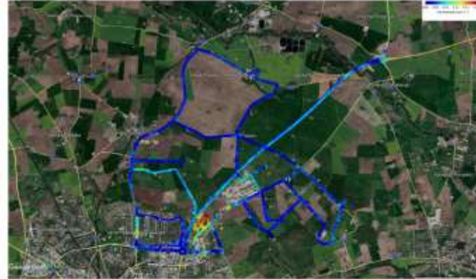
Figure 4 Mobile (car) gamma spectroscopy (NaI(Tl)) around ESS in August 2020. The colour scale shows the average dose rate ( \mu\text{Sv h}^{-1} ) as detected by the NaI(Tl) detectors, averaged over one second, from blue ( 0.06 \mu\text{Sv h}^{-1} ) to red ( 0.17 \mu\text{Sv h}^{-1} ). Although within normal background levels for the area, the highest values observed are due to naturally occurring radionuclides in nearby soil piles and buildings.
